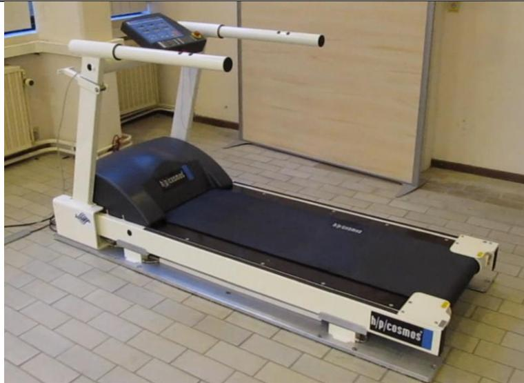
The gaitway-3D is an instrumented treadmill designed by h/p/cosmos and Arsalis. The system shown here is optimized for walking and slow speeds of running.
