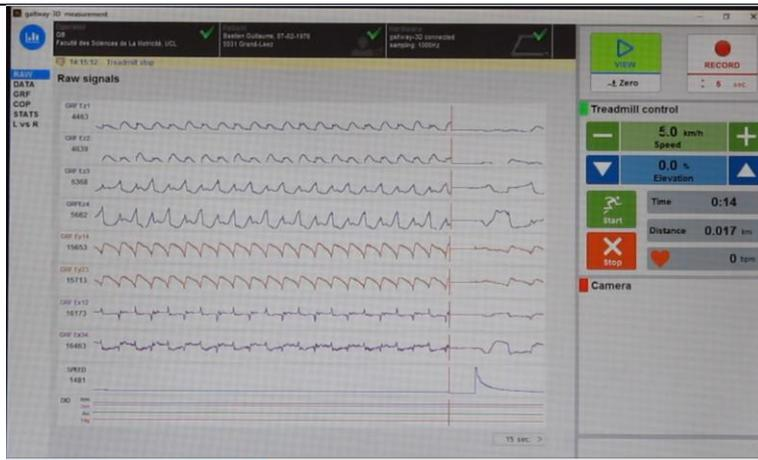
The treadmill can be controlled from any screen during the measurements. The software allows the control of the treadmill speed and elevation and it also reports the exercise time, distance and heart rate. The first panel shows the raw data, in bits, as they are sampled from the A to D converter. This includes 8 force signals, one treadmill speed and 4 digital signals. The data monitoring can be started and stopped at any time via the "View" function.
