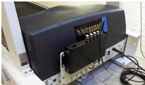
The load cells are mounted to a dedicated frame that is bolted to the floor. This ensures an optimal rigidity and an optimal signal quality. The 3D amplifier mounted at the front delivers the signals to the software via an Ethernet interface.
