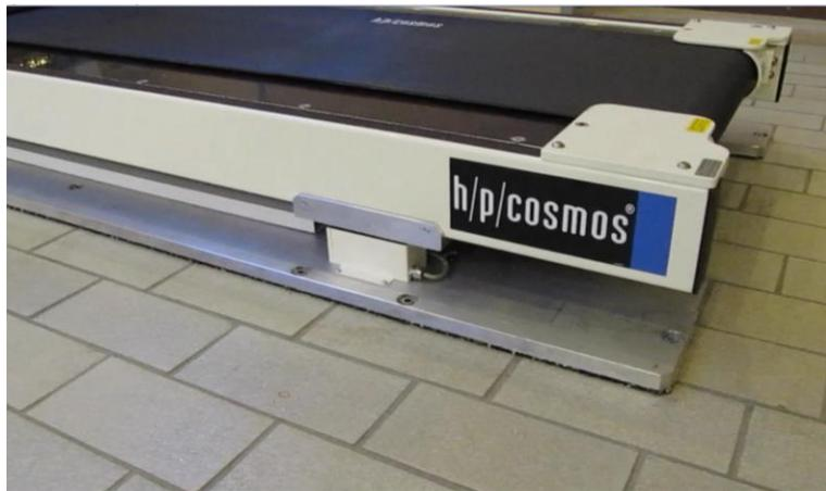
The treadmill feet and elevation system are replaced with tree-dimensional load cells that can measure forces up to 1 Ton in each direction.
